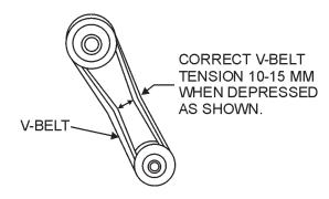
Figure 9. V-Belt Tension
